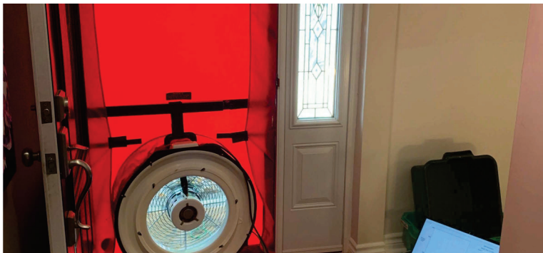
Blower door testing to assess baseline of air tightness
