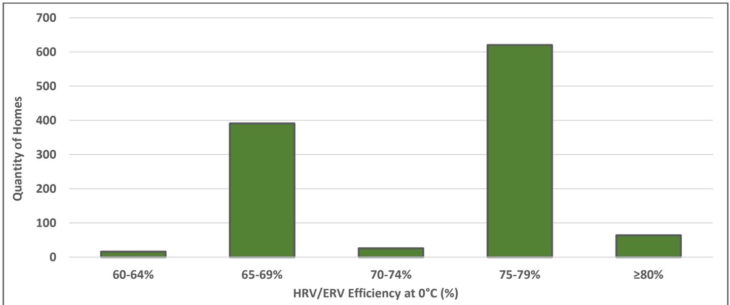
Figure 10: HRV/ERV Efficiency at 0°C
