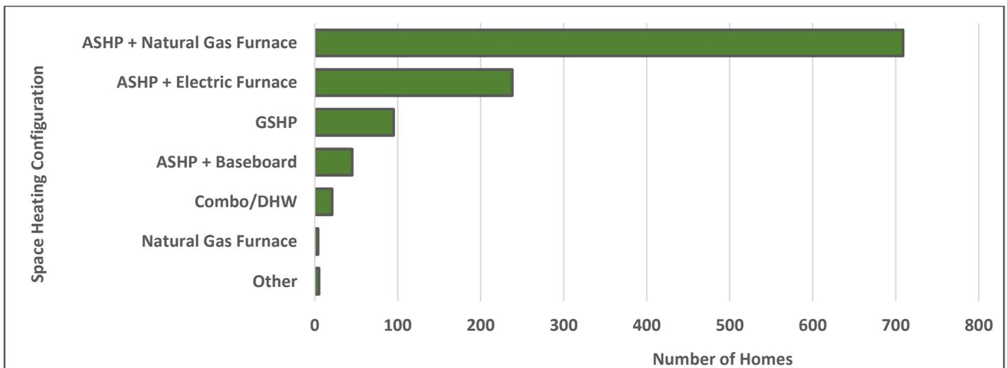
Figure 8: Space Heating Configuration
